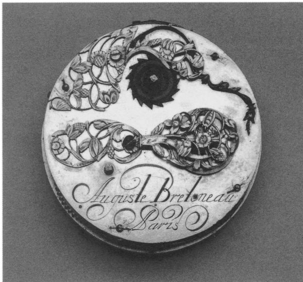
Figure 30. Auguste Bretonneau (French, recorded 1638–58). Movement of the watch in Figure 17. Gilt brass; steel, partly blued; and silver, diam. of back plate 1 \frac{1}{4} in. (4.4 cm)
